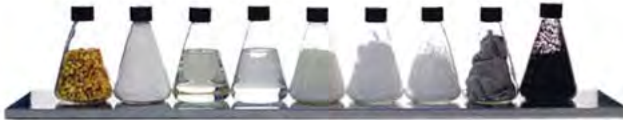
Corn Starch Dextrose Lactide PLA Ingeo Yarn Kira Compost
